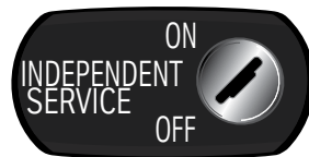
Independent service keyswitch Elevator no longer responds to hall calls and remains on a floor with its doors open until a floor is selected and the "Door Close" button is held; then, the elevator starts to travel. Useful when transporting large goods or moving groups of people between certain floors. Key L203
