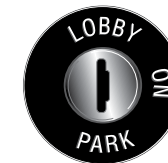
Lobby park keyswitch Brings car to designated floor and shuts down car operation. Key L206
