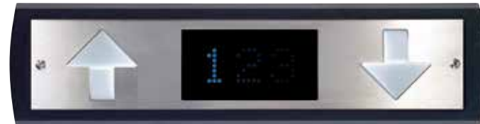
Combination hall lantern and position indicator Illuminated numbers or letters indicate the position of the elevator. Up and down arrows indicate which direction the elevator will travel when leaving the floor. A tone sounds once if the elevator is traveling up, twice if going down.
