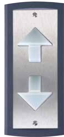
Hall lantern Up and down arrows illuminate, indicating which direction the elevator will travel when leaving the floor. A tone sounds once if the elevator is traveling up, twice if going down.
