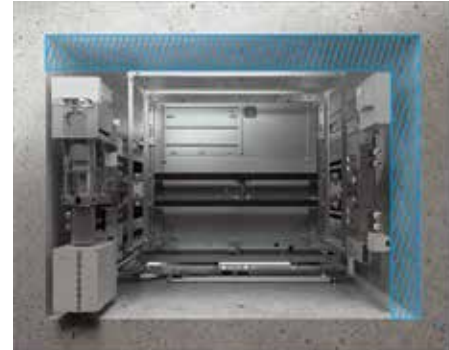
Reduced hoistway width, depth and height are due to the compact machine with small components and underslung design. This results in a smaller building footprint.
